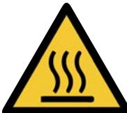
Warning; Hot Surface
