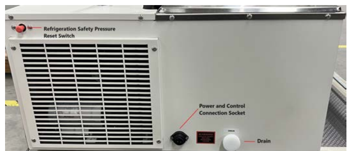
Fig 2. Refrigeration safety pressure switch location
