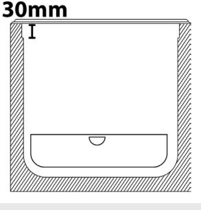
Fig 2. Maximum fill level.
