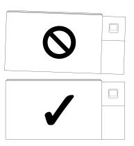
Ensure the bath is placed on a level surface.
