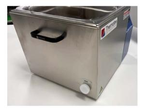
To drain the bath simply find the drain located on the side of the bath and pull it out (exposing the hose). You can then remove the plug to drain the water.
