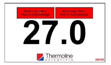
**NOTE:** You must log into the main screen to mute and acknowledge alarms. Alarms can only be acknowledged once the condition has returned to a non alarm state.
