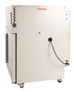
Once the TPS-18 has been placed inside, pull the excess cable back out through the 54mm port hole. This will reduce the risk of the TPS-18 fouling on either cable while in operation.
