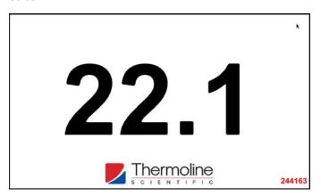
To exit the screen saver, you will need to input the security code. Press the Thermoline logo, as shown below, to access the passcode.
