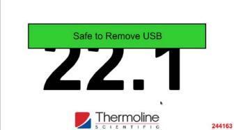
Once the data has been downloaded, the STAR X controller will notify you that it is safe to remove the hardware, as shown above.
