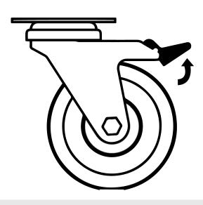
Fig 3. Castor Unlocked
