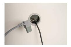
Power down the TMLR-200 before installing the TPS-18. Plug the power lead into the port on the side of the TMLR-200 and feed both leads through the 54mm port hole. Using a trolley, bring the TPS-18 close to the open door of the TMLR-200 and connect the power and BMS leads. Carefully slide the TPS-18 into the TMLR-200.
