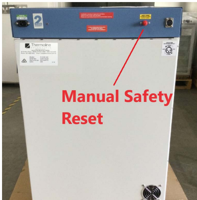
Fig 1. Manual Safety Reset 145
