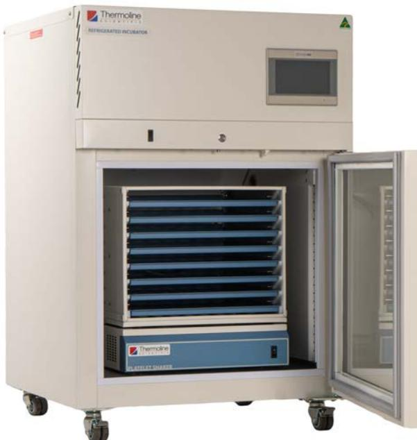
Turn the TMLR-200 back on and start the agitation on the TPS-18. The heat generated by the TPS-18 helps control the internal temperature of the refrigerated incubator, so it should be left on at all times other than when it is being loaded with samples.
