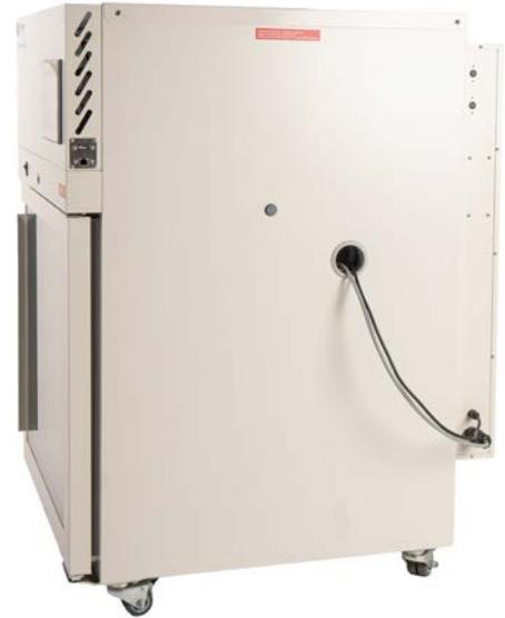
Once the TPS-18 has been placed inside, pull the excess cable back out through the 54mm port hole. This will reduce the risk of the TPS-18 fouling on either cable while in operation.
