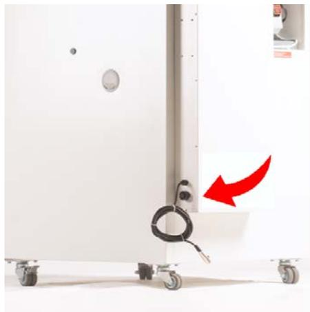
Supplied with the TMLR-200 is a power lead to connect the TPS-18 to the incubator. On the TMLR-200, there is a lead to connect to the special socket for BMS on the TPS-18. Both of these leads go through the 54mm port hole on the side of the TMLR-200.
