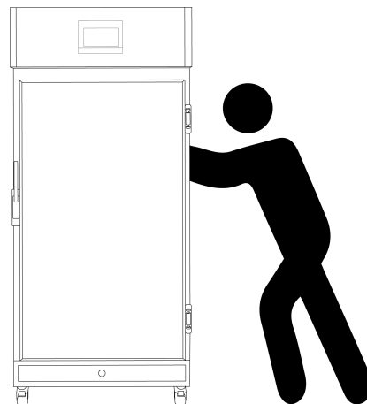
Fig 3 . Safe moving of cabinet.
