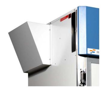
When installing more than one Humiditherm or Envirotherm cabinet ensure that they are positioned in such a way that the air from the ventilation grill from one cabinet, is not directly drawn into the ventilation grill of the next cabinet. If adequate spacing cannot be achieved then deflectors can be used to direct the hot air away from the adjacent cabinet.
