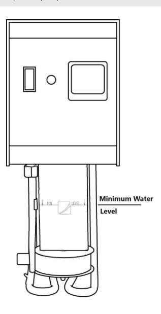
Fig 1. Minimum fill level.
