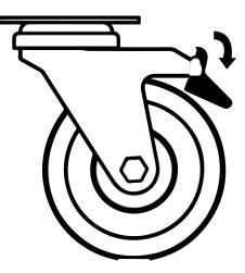
Fig 3. Castor Locked
