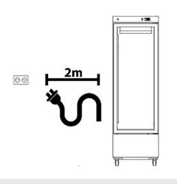
Fig 1. Suitable distance from power supply (2m)
