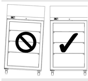
Fig 1. Correct Levelling
