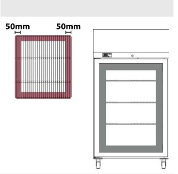
Please ensure that the highlighted areas are free to allow air to pass and that the samples on the shelves allow air to pass between them.
