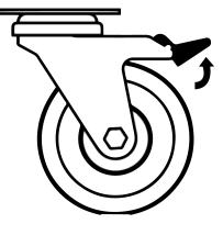
Fig 2. Castor Unlocked
