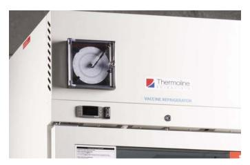
A circular chart recorder can be factory fitted as an optional extra. The recorder has a seven day chart with a battery backup that will keep the chart running for at least 24 hours in the event of a power failure.
