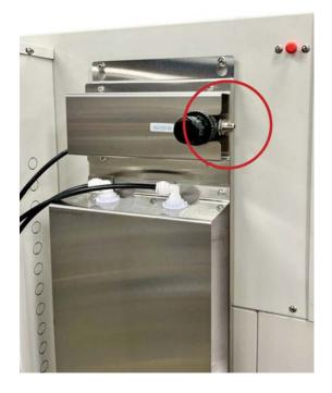
Fig 6. Water Pressure Regulator Connection
