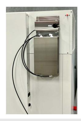
Fig 3. Installed Water Filter
