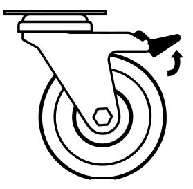
Fig 3. Castor Unlocked
