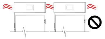
Fig 2. TEC cabinets transferring heat to another cabinet reducing performance.
