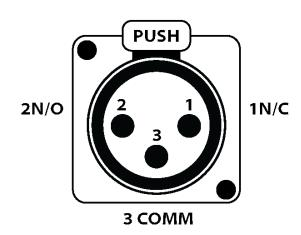
1N/C: Will open loop upon alarm situation. This is the optimal option, as any break in the loop is detected.
