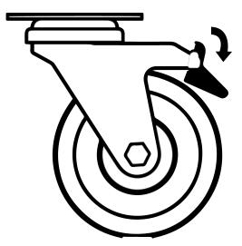
Fig 2. Castor Locked
