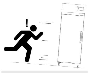
Fig 1. Castor Unlocked
