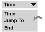
After selecting the Jump To parameter, you must change the values in the two sections below. The first section, labelled 'Jump To' determines which segment the cycle is repeated from, and the 'Jump Cycle' parameter determines how many times the cycle is repeated.
