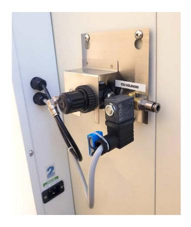
Fig 1. CO<sub>2</sub> connection
