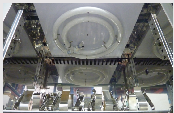
Inside: Circular fluorescent lighting on the chamber roof.
