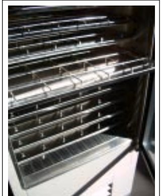
• Perforated stainless steel shelves with wire grid support to easily separate cement test samples.
