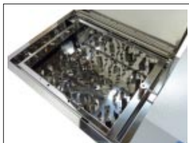
Shaking water bath shown with the standard flat tray and flask clips. Flask clip sizes available: 50ml, 125ml, 250ml, 500ml and 1000ml
